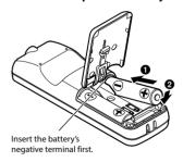
3 Slide the battery cover completely closed.
