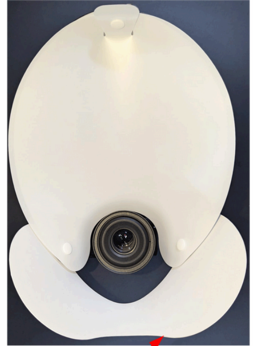
Reflector Panel Installed at the Bottom
