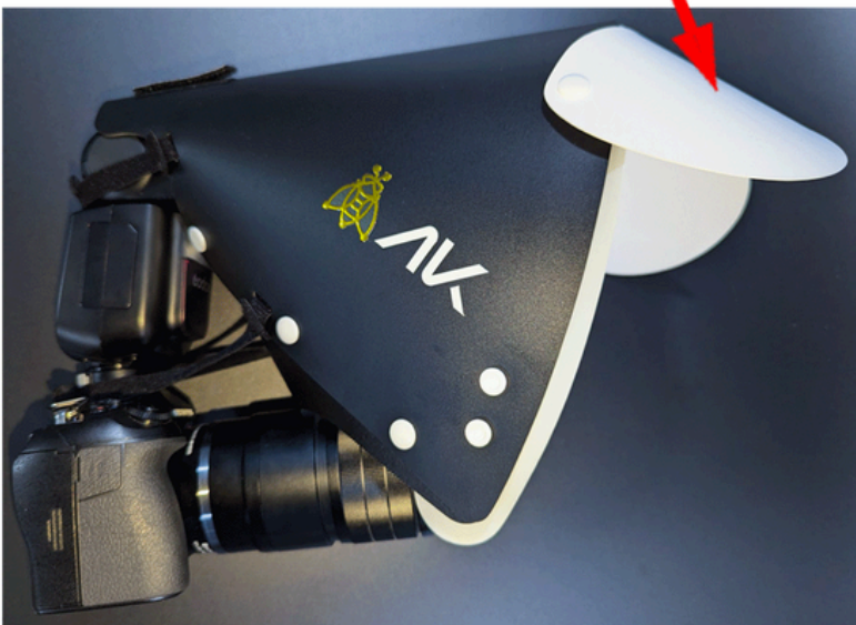
Reflector Panel Installed at the Top
