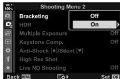
Combine multiple images for a depth of field greater than can be obtained with a single shot. The camera takes a series of shots at focus distances both in front of and behind the current focus position and creates a single image from the areas that are in focus in each shot.
