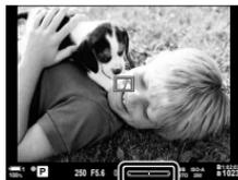
Display when shutter button is pressed halfway
